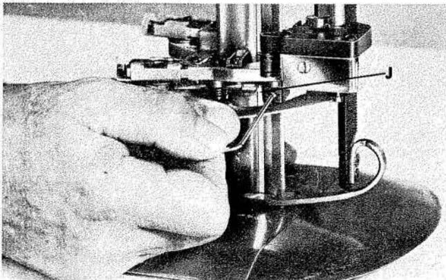
mally an acceptable bevel is 1/16" wide. If necessary to adjust the bevel on the knife edge to a different length proceed as follows:
