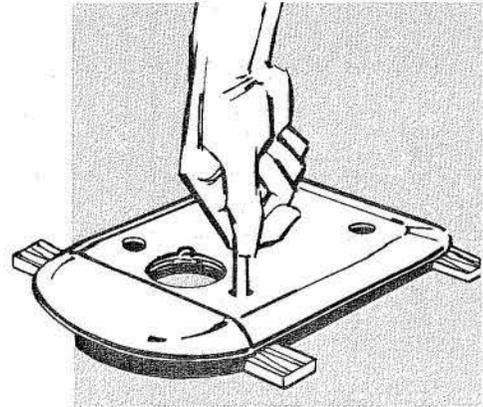
Place plate on blocks and press out roller shell from ring assembly, as shown.
